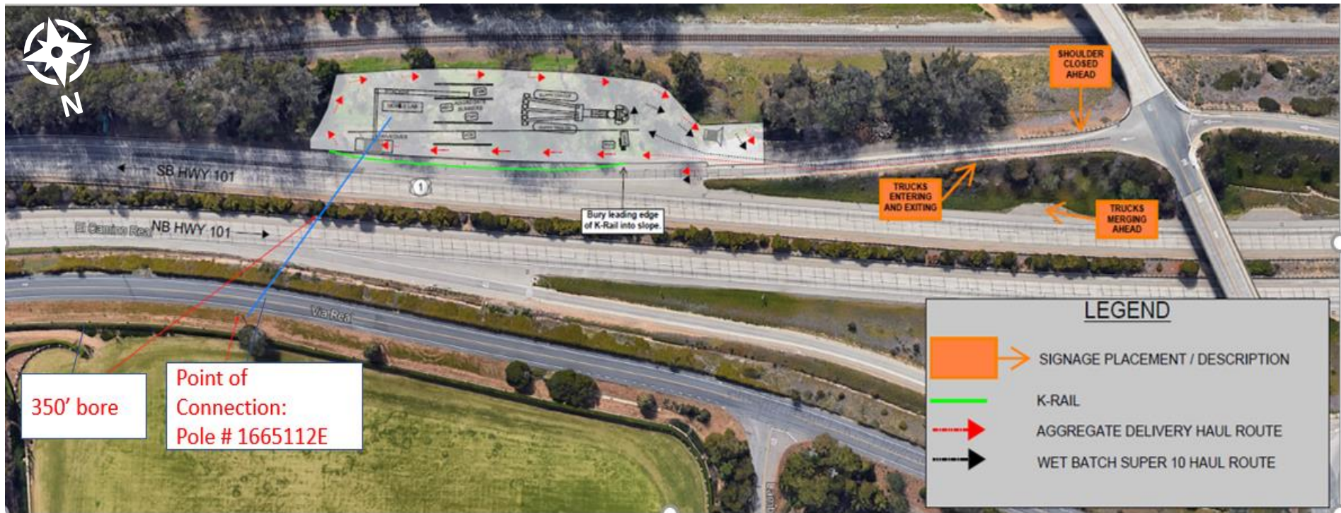
Figure 1 – Boring Location for Electrical Power Connection at Construction Support Site
