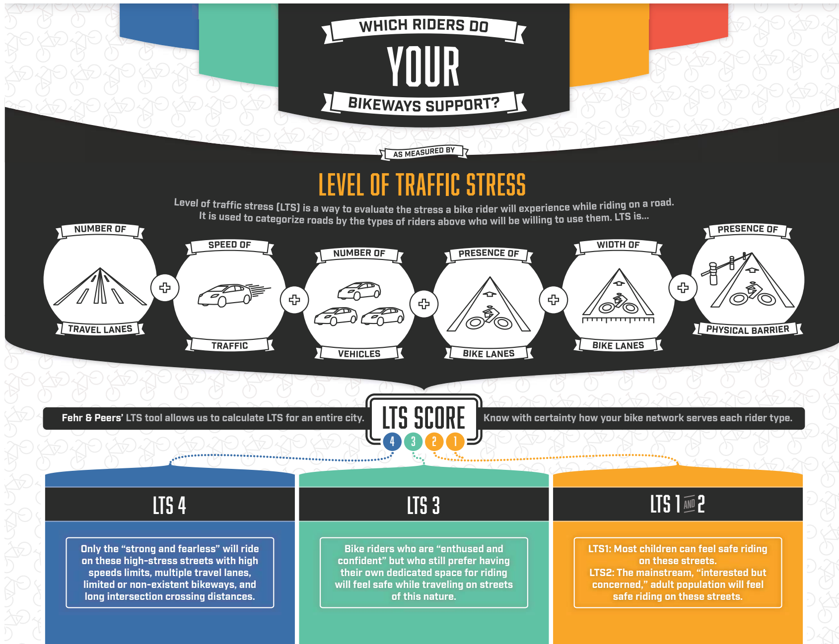
Figure 3-3. Level of Traffic Stress
